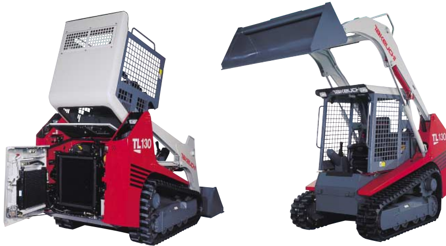
Tilt-Back Operator's Compartment for Easy Service Access
