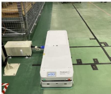
AGV (runs on a magnetic guide)
