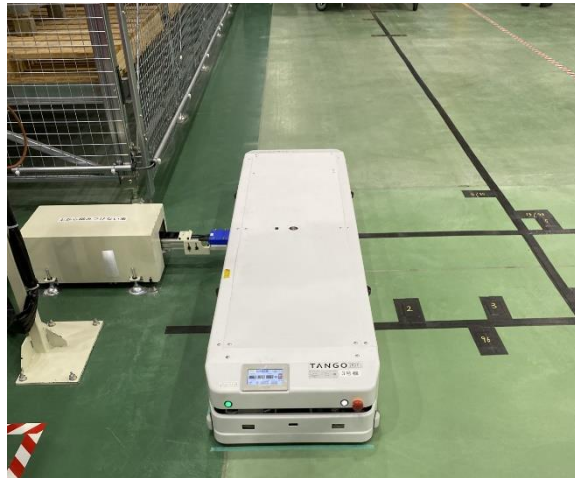
AGV (runs on a magnetic guide)
