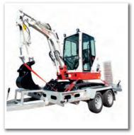
provides plenty of room for extras in the trailer: attachments, breakers, buckets or materials with added tie down points, whilst still being able to transport it from site to site on a standard UK licence. The power is significant on the TB225, with a Yanmar 3-cylinder engine providing more than 16.5 kW/2,200 rpm. That's massive in this weight class and just
